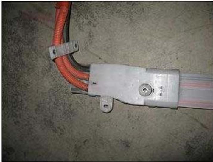
*(6) Examples of DC Orange Wires from Battery to Inverter (Note AC Orange Wires on Top of Traction Motor)*
