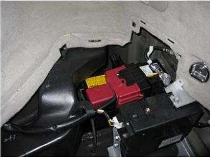
*(8) Prius 12V Battery - Located in RH Rear Corner of Vehicle (Note red plastic cover over the “+” battery terminal)*
