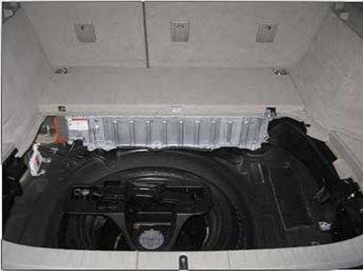
(1) Examples of a Prius High-Voltage Battery. (Note location of battery under floor, behind rear seat)
